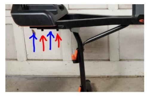
Line the stand leg gusset tubes (red arrows) up with the holes in the base (blue arrows). Please note this pilot model has shorter gusset tubes than the models in production. This has no effect on assembly.
