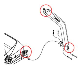
The cable connections to check are circled in red.
