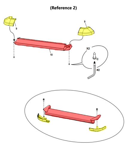
The front platform frame is highlighted in red with the coordinating corner pieces highlighted in yellow.
