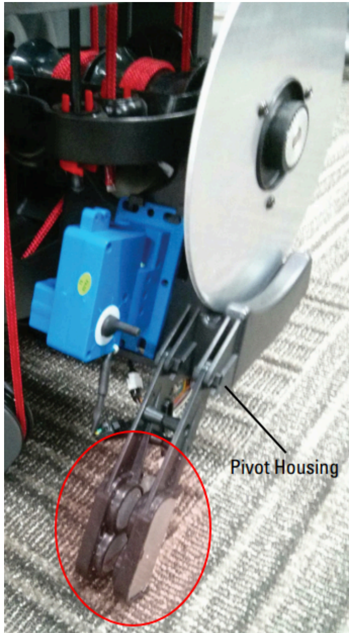
A more detailed view of the magnets in the brake arm, all magnets should be present.
