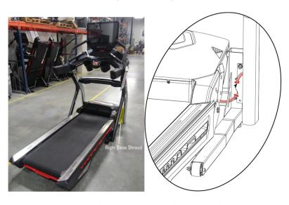
Treadmill 22 shown. Your treadmill may vary slightly. Remove the right base shroud to access the 5-pin connector.
