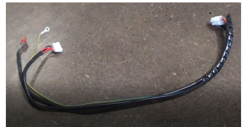
The Lower I/O Cable with multiple connectors.
