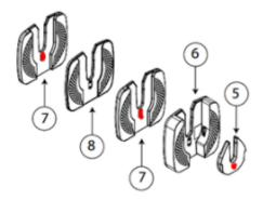
The red markings indicate the position of the selection tabs. The weight plates are installed with the 1.25 lb plate closest to the handle, followed by the 13.75 lb plate, 5 lb plate, 2.5 lb plate, and another 5 lb plate.
