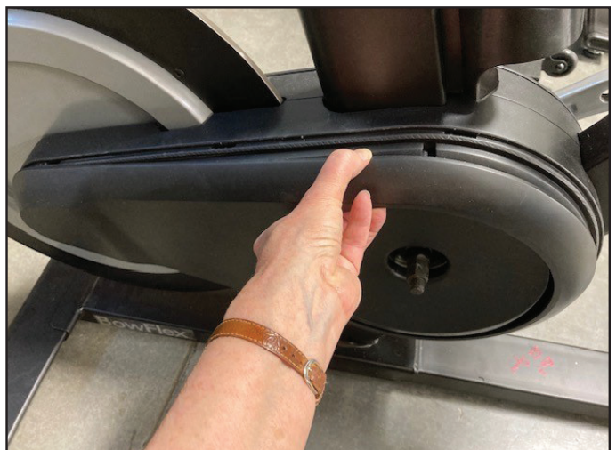
Removing Right outside shroud (Crank arm not shown)
