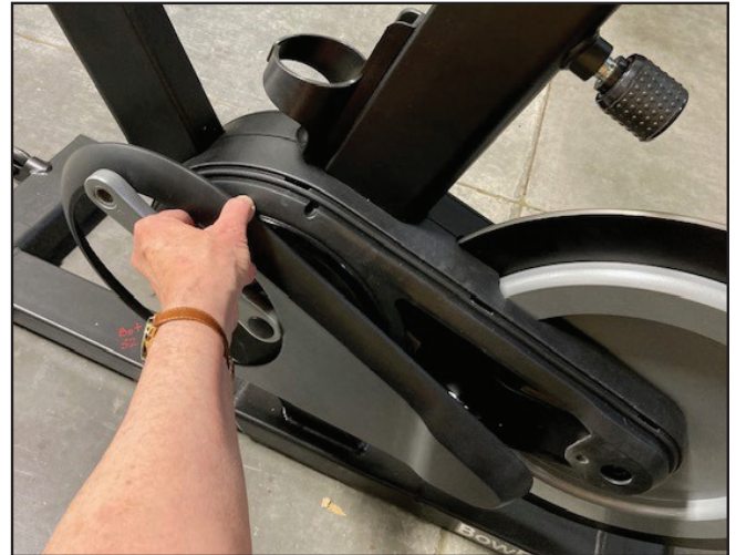
Removing left outside shroud (Pedal not shown)
