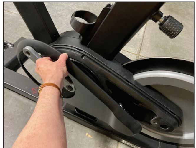
Removing left outside shroud (Pedal not shown)
