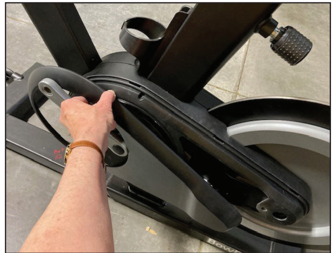
Removing left outside shroud (Pedal not shown)
