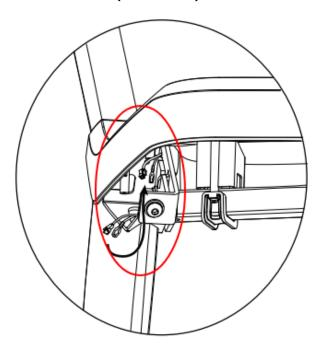
The cable connections to check at the top of the upright are circled in red. You can access the cables from the rear of the console.
