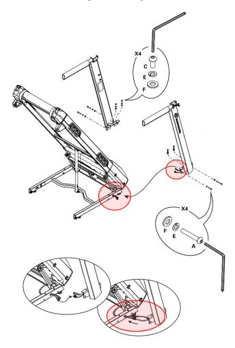
The cable connections to check at the bottom of the upright are circled in red.
