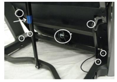
Use the wrenches from the tools list above to tighten the circled hardware.
