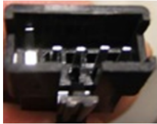
An example of a damaged connector with a bent pin.
