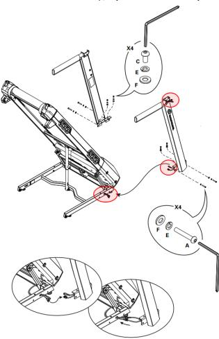
The cable connections to check are circled in red.
