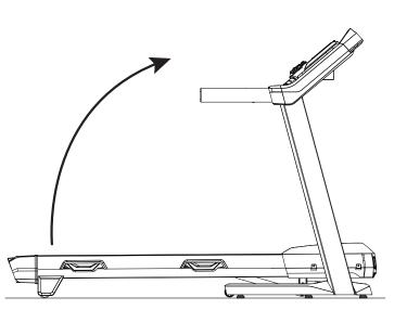
7. Make sure that the locking mechanism is engaged. Carefully pull back on the walking deck and make sure that it does not move. When you do this, keep clear of movement path in case the treadmill lock is not properly engaged.
