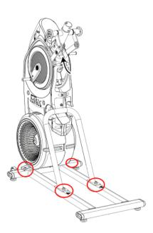
The red circles in this image indicate the location of the 4 larger bolts to tighten on the base assembly.
