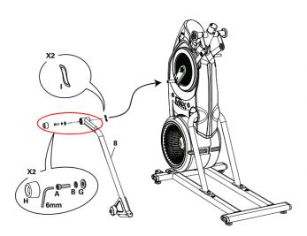
The Wave Washers are the part labeled 'I' in this image. These should be installed between the crank arm and the pedal arm (8).
