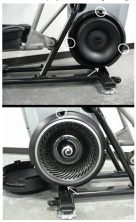
The top image indicates the locations of the screws for the lower right fan cover. Remove the screws in the white circles and loosen the screw at the white arrow. Unplug the power inlet wire and then remove the cover.
