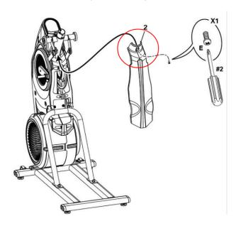
The screw to remove is circled in red. Once removed, the rear shroud can be removed as well.
