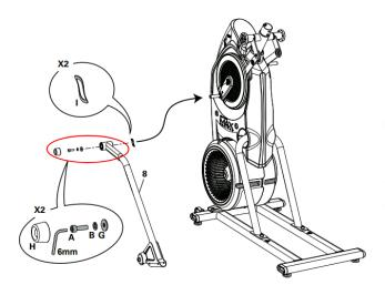
The cap is the part labeled 'H' in this image. Remove the cap and loosen the screw (A) using a 6mm Allen wrench.
