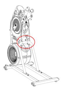
The red circle in the center of this image indicates the location of the first 4 bolts to tighten on the rail assembly and frame.
