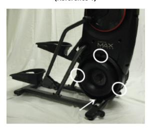
The white circles indicate the locations of the 3 upper screws to remove. The white arrow indicates the location of the power plug inlet wire and bottom screw. Loosen the bottom screw by at least 3 turns, unplug the power inlet wire, then remove the cover.
