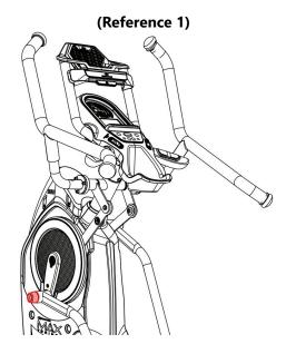
The end cap (highlighted red) is the small rubber component located at the pedal arm and crank arm connection.
