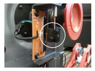
The white circle indicates the location of the screws to loosen in order to adjust the position of the black plastic bracket.
