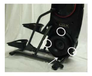
The white arrow indicates the location of the power plug wire inlet and bottom screw. The bottom screw can be loosened 3 turns rather than removing it entirely. The white circles indicate the locations of the screws to remove in order to remove the cover.
