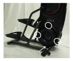
The white circles indicate the locations of the 3 upper screws to remove. The white arrow indicates the location of the power plug inlet wire and bottom screw. Loosen the screw by at least 3 turns, unplug the power inlet wire, then remove the cover.
