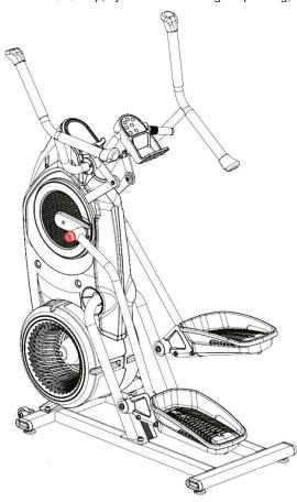
The end cap (highlighted red) is the small rubber component located at the pedal arm and crank arm connection.
