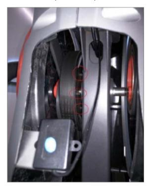
The red circles in this image indicate the locations of the pulley screws on the drive pulley. The foot pedals can be used to rotate the pulley, allowing all 4 screws to be inspected.
