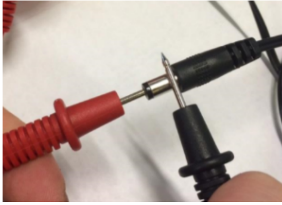
This image shows the proper positioning of the voltmeter on the connection.
