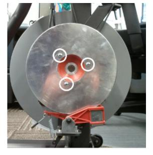
The white circles indicate the locations of the screws to remove in order to remove the brake disc.
