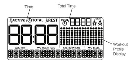
TOTAL: During a Manual workout, the TIME display will count up until the workout is ended.
