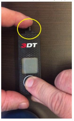
The plunger, circled in yellow, should be able to move freely when pressed.
