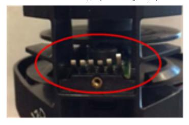
The red circle shows the sensor contacts on the handle. The rightmost contact is bent out of place and should be gently corrected.
