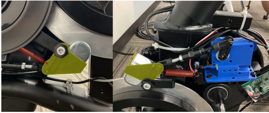
The magnet carriage return spring is located between the resistance magnets and servo motor (left Schwinn 190; right Schwinn 290). The spring (highlighted red) should be attached to the magnet carriage (highlighted yellow) as shown above.
