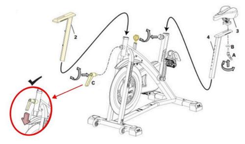
The Handlebar Post (2) should be inserted into the frame with the Handlebar Post Adjustment Knob engaged in the holes of the post. The handle on the knob should be pointed downward once completely tightened.
