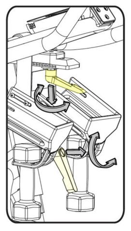
The Handlebar Adjustment Knob is located directly underneath the handlebars. The Handlebar Post Adjustment Knob is located on the front of the bike between the dumbbell holders.
