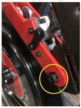
The hardware to loosen is circled in yellow. Use the 10mm wrench with the Allen wrench in reference 5 to loosen the hardware.
