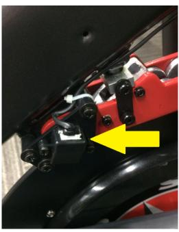
This image shows the location of the Resistance Sensor. It is located on the user's right side of the bike
