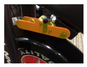
Schwinn IC4 pictured. Functionality is the same, but your bike may vary slightly. The red magnetic brake arm (highlighted yellow) is located above the flywheel. Watch this part for movement while adjusting the Resistance Adjustment Knob.
