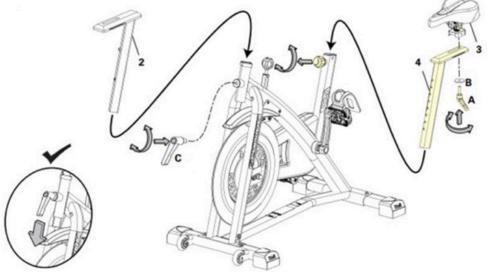
The Seat (3) should be secured onto the Seat Post (4). Tighten the Seat Adjustment Knob (A) by turning the handle clockwise until fully tightened. Tighten the Seat Clamp Bolts using the 15mm/17mm wrench included with your machine until fully tightened.
