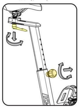
The Seat Adjustment Knob is located underneath the Seat. Turn the handle clockwise to tighten the Seat.
