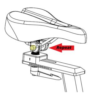
The Seat Clamp Bolts are located underneath the seat, on either side of the seat's stem.
