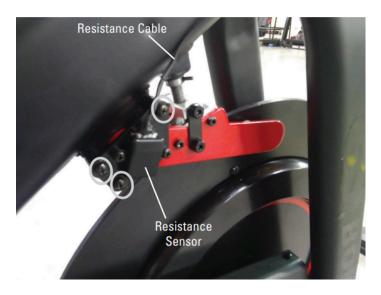
The resistance sensor and sensor cable are identified above.
