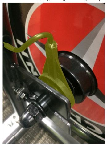
The Speed Sensor is located in the center of this image, sandwiched between the flywheel and the frame bracket.
