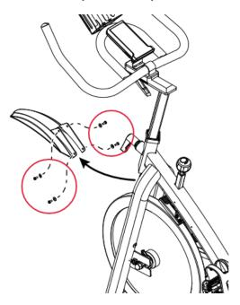
The fender is attached to the frame by 4 screws, shown on the left side of the image circled in red.
