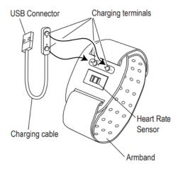
The optical sensor is the clear window located in the center of the underside of the monitor, just below the charging terminals
