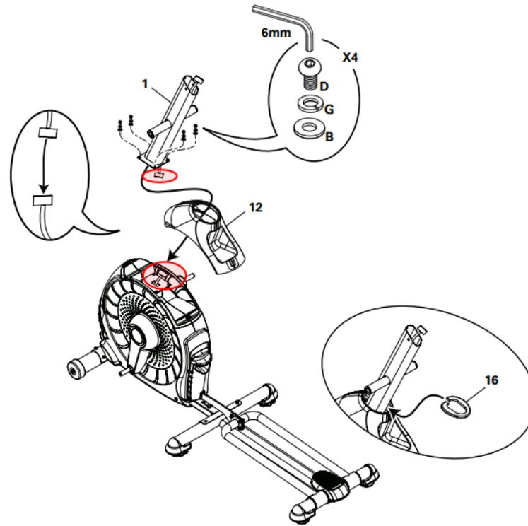
*Inspect the 12-pin cables circled in red for damage.*
