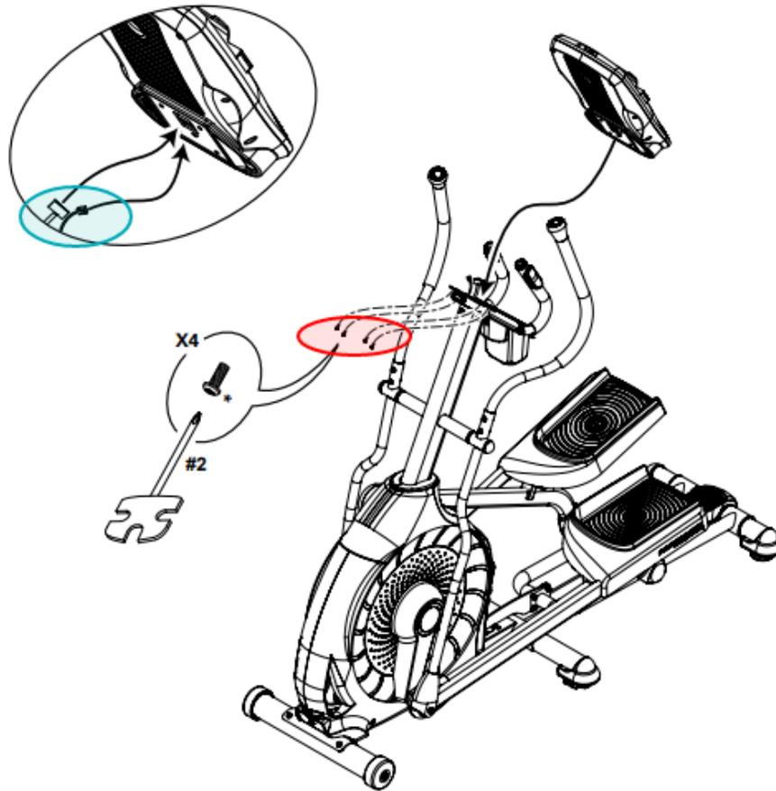
*The bolts circled in red need to be removed to access the cables between the console and the console mast.
