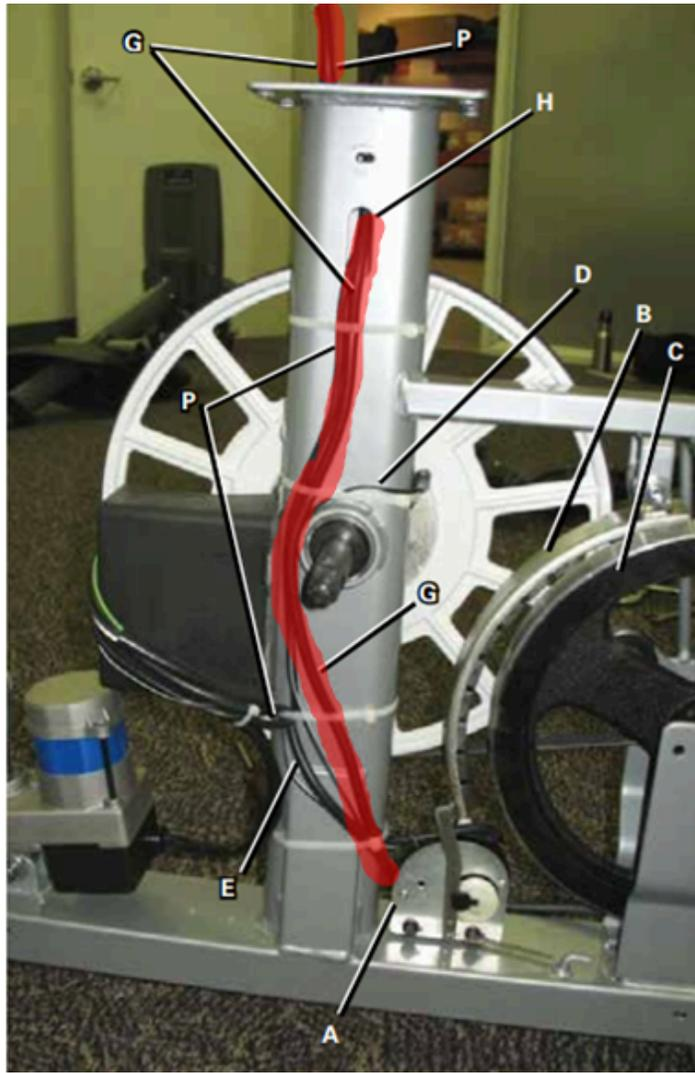
*The mast to servo cable is highlighted in red and the servo motor is labeled 'A.'
