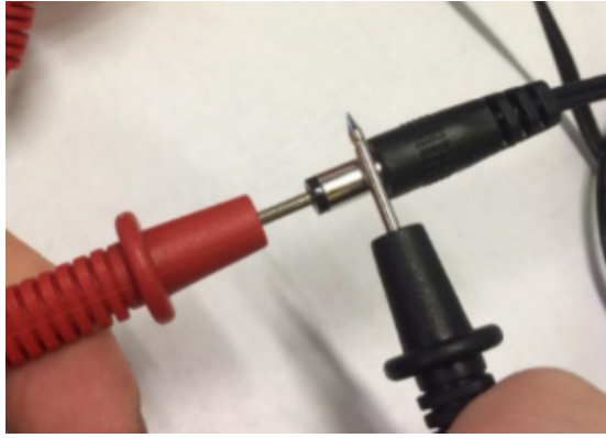
This image shows the proper positioning of the voltmeter on the connection.
