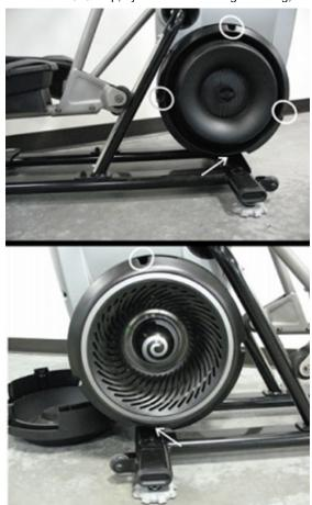
The white circles and arrows indicate the location of the screws to remove in order to remove the lower fan covers. For the lower right fan cover, only the upper 3 screws need to be removed. Loosen the bottom screw by at least 3 turns, unplug the power inlet wire, then lift and remove the cover.
