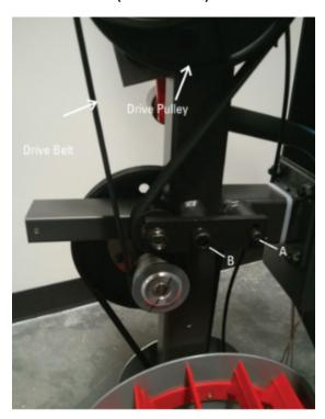
White arrows indicate the location of the drive belt and pulley. White lines indicate the location of the A and B screws on the tensioner arm.
