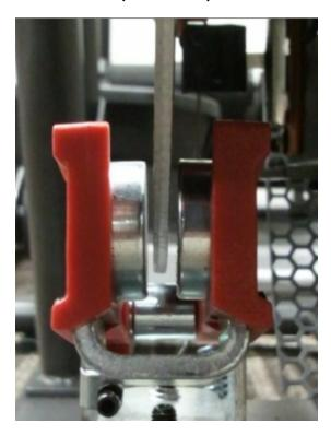
When brake magnets are distanced from the brake disc properly, they should appear the same as in this photo.
