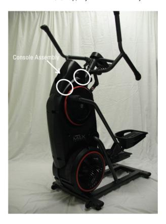
Remove the screws circled in white, then remove the console hood.
