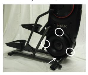
The white circles indicate the location of the 3 upper screws to remove. The white arrow indicates the location of the power plug inlet wire and the bottom screw. Loosen the bottom screw by at least 3 turns, unplug the power inlet wire, then remove the cover.
