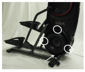
The white circles indicate the location of the 3 upper screws to remove. The white arrow indicates the location of the power plug inlet wire and bottom screw. Loosen the bottom screw by at least 3 turns, unplug the power inlet wire, then remove the cover.
