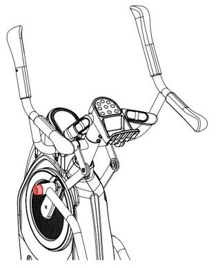
The end cap (highlighted red) is the small rubber component located at the pedal arm and crank arm connection. There is no hardware connecting the end cap, just pop it off to remove.
