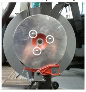
The white circles indicate the locations of the screws to remove in order to remove the brake disc.
