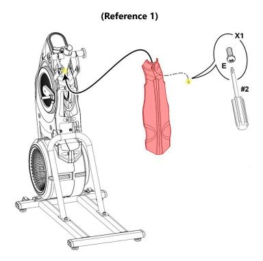
This image shows the location of the rear tall plastic cover and the location of the screw to remove it from the machine.
