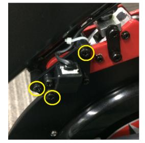
The three yellow circles indicate the location of the screws to remove in order to access the Resistance Sensor Magnet.
