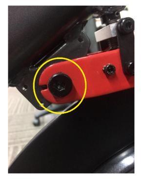
The hardware to loosen is circled in yellow. Use the 5mm Allen wrench with the open-ended wrench in reference 4 to loosen the hardware.
