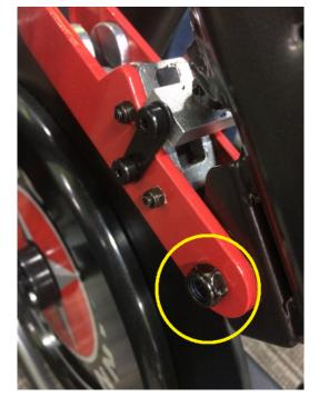
The hardware to loosen is circled in yellow. Use the 10mm wrench with the Allen wrench in reference 5 to loosen the hardware.
