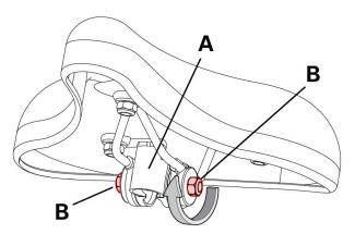
Tighten both seat clamp nuts (B, highlighted red) to secure the seat to the seat post. Image may not match your bike exactly - the BowFlex C6 is shown in this image.
