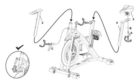
The Seat (3) should be secured onto the Seat Post (4). Tighten the Seat Adjustment Knob (A) by turning the handle clockwise until fully tightened. Tighten the Seat Clamp Bolts using the 15mm/17mm wrench included with your machine until fully tightened.
