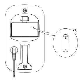
The Console display will show "Batt" during power up if the battery level is low. When replacing the batteries, make sure the batteries point in the +/- direction shown in the battery bay.
