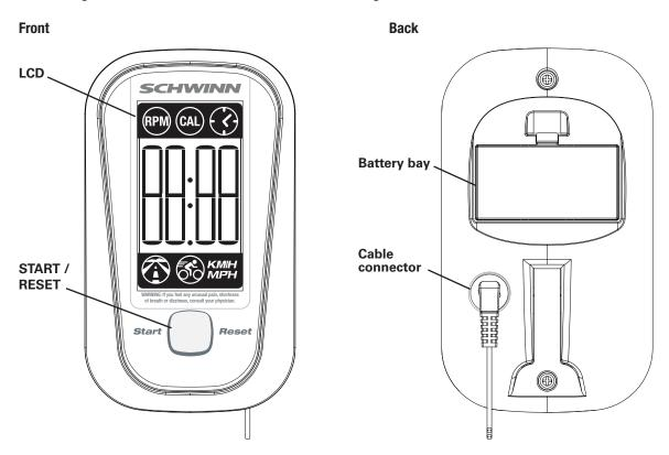
START/RESET Push to start, or to stop an active workout and reset the Time to 0:00.
