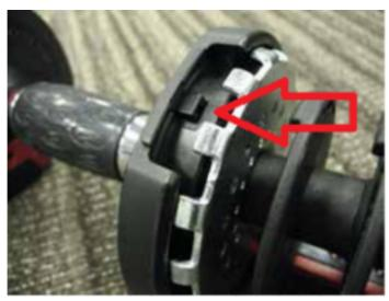
The red arrow indicates the location of the locking mechanism button.
