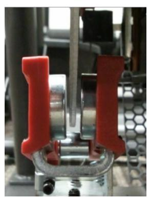
When brake magnets are distanced from the brake disc properly, they should appear the same as in this photo.
