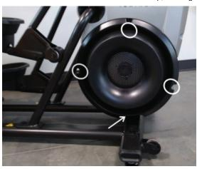
The white circles indicate the location of the 3 upper screws to remove. The white arrow indicates the location of the power inlet wire and the bottom screw. Loosen the bottom screw by at least 3 turns, unplug the power inlet wire, then remove the cover.
