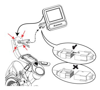
Remove the 4 screws at the locations indicated by the red arrows. Rest the console on the handlebar tray, just above the resistance adjustment knob. Check each connection and orient them as shown.
