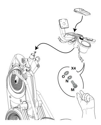
Use a 5mm Allen wrench to remove the two front and two rear bolts at the engine/handlebar connection.
