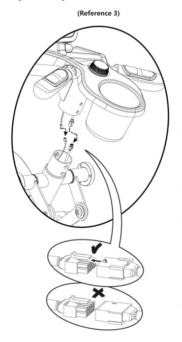
Make sure that the cables are undamaged, oriented properly as shown, and connected securely.
